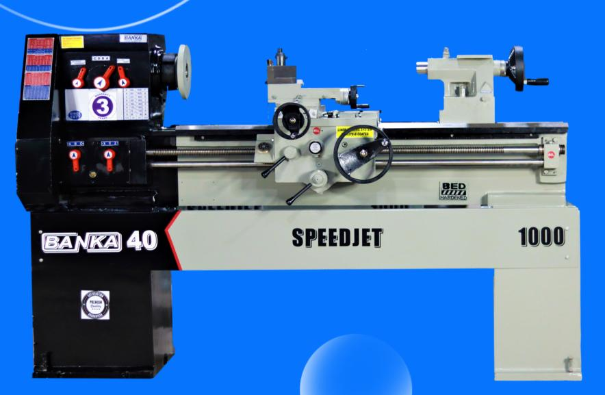
Height Of Center: 200 mm Spindle Bore: 51 mm Admin Between Center: 1000/1200 mm Spindle Speed: 1535 RPM Bed Width: 280 mm Cross Slide Travel: 210 mm Motor : 3HP
